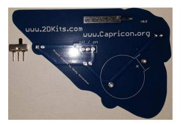
2. Flip the board over and solder the pinback. It will take a bit more time to heat up, so hold the soldering iron firmly against the base of the pinback and wait for the solder to flow.
