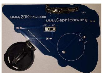
4. Flip the board over. Insert the battery. The plus sign "+" will face up. Angle it into the battery holder on the left side first, and then press down. It will snap in place. Verify the power switch is on. In the next few steps, the LEDs will be inserted and tested before they are soldered into the board.
