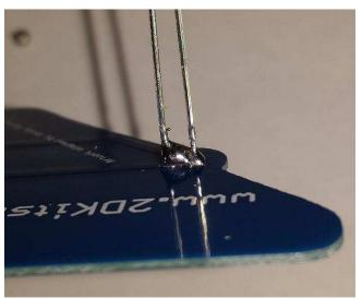
Needs to be fixed: A bridge between the two leads of the LED. Current will flow through the bridge, and not the LED, thus the LED will not light up.
