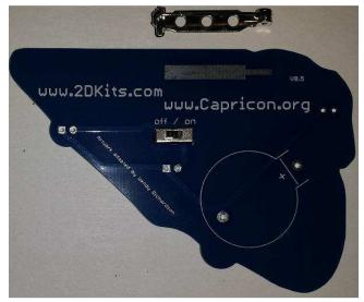
3. Insert the battery holder. Remember, orientation is important for the battery holder. Make sure the battery holder matches the printed outline. Flip the board over to the GOAT side. Solder the battery holder.
